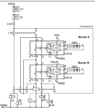
With this type of supervision, too, the burner can be started only if the flame detector or flame simulation test has been successful.
