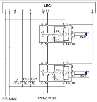
With this type of supervision, **1** flame is supervised by **2** independently operating flame safeguards, aimed at reducing the possibility of loss of flame during operation in case of a simultaneous failure of **both** flame safeguards to an «improbable coincidence».
