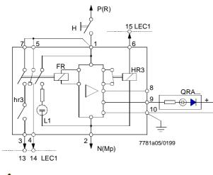
Terminal 10 must be connected to earth!
